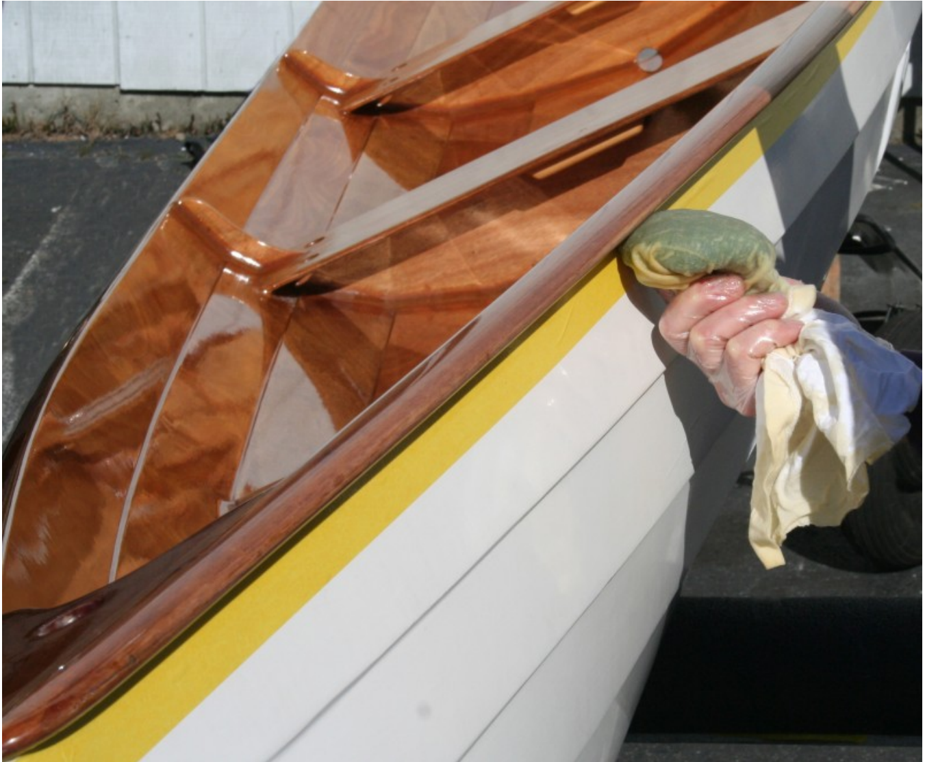
With masking tape protecting the painted hull, Don can move with the speed necessary to wipe on the thinned varnish.
