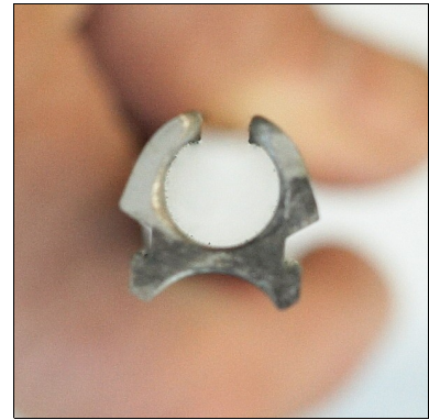
Rear section of spar
