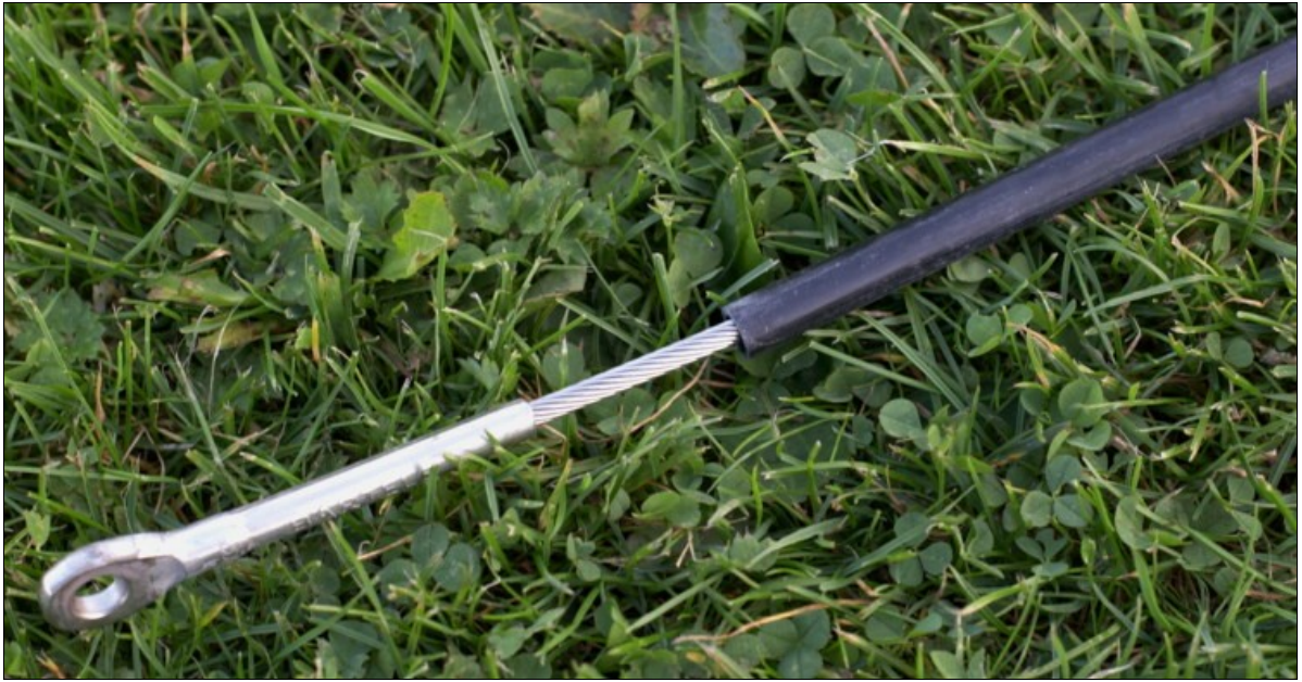
Top of forestay, showing plastic sleeving (slid back for photo)
