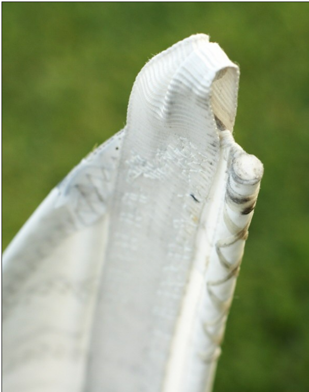
Genoa bolt rope and tape loop
