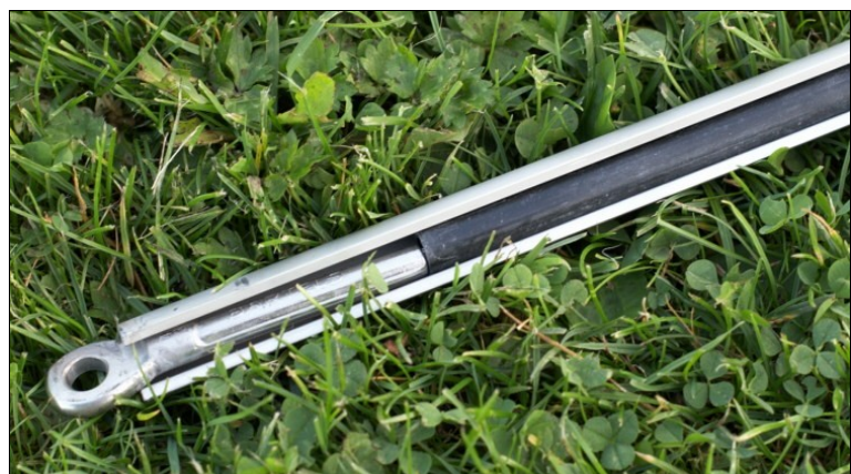
Forestay in spar, showing plastic sleeve
