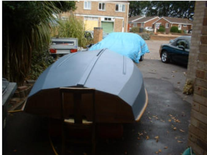
measurement form), then just a few hundred screw holes to fill, scarf-joints to fill and fair-in. Epoxy coating, undercoats, top coats metal rubbing bands....
